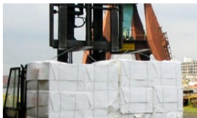
... unsuitable lifting with fork tip
