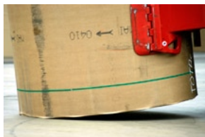
Edge damage due to lowering at an angle
