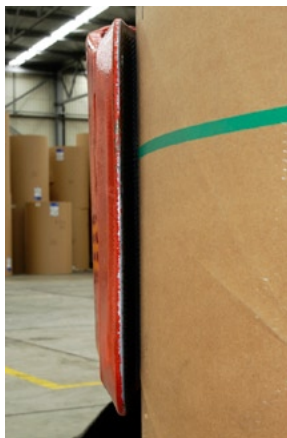
„Gap“ between contact plate and reel
