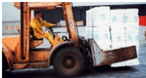
Badly clamped pulp units
