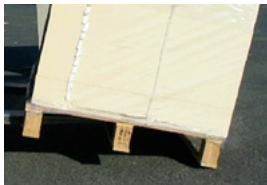
Mast tilted, foot breaks off
