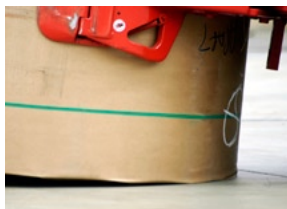
Edge damage due to lowering at an angle
