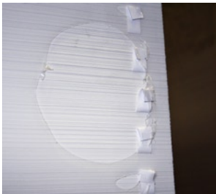
Holes in shrink wrapping
