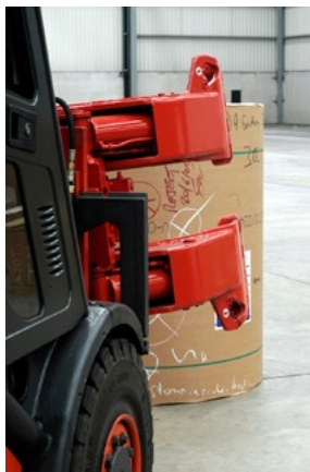
Clamp not in zero degree position
