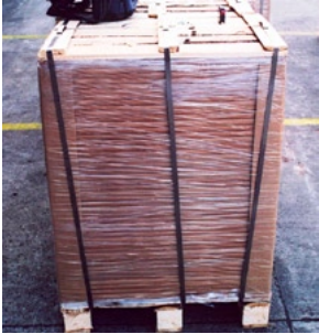
Pallet with paper in sheets with quintuple strapping
