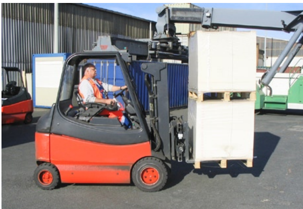
Danger of tilting if truck has to brake sharply
