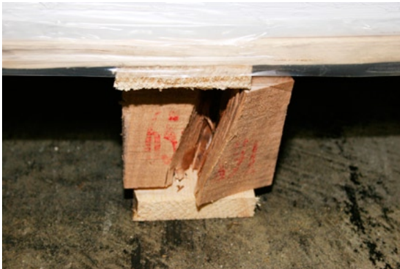
Damaged pallet foot
