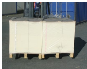
Double pallet lifting
