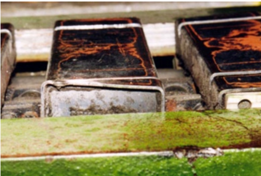
Faulty section of a slat conveyor for paper reels
