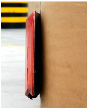
Contact plate not resting fully against reel
