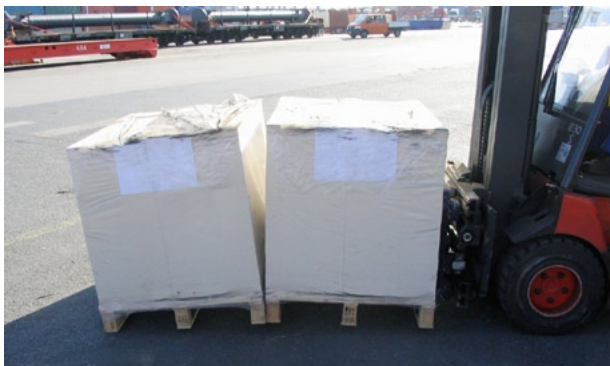
Pallet feet threaten to break off during transport
