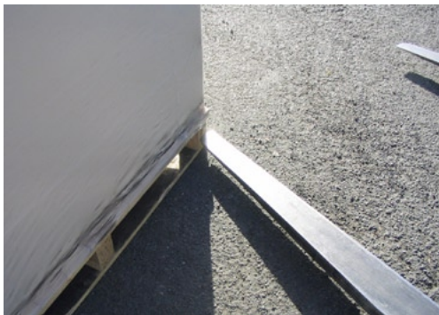
Pallet foot is damaged
