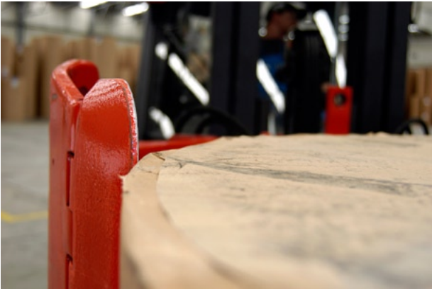
Contact plate can damage reel
