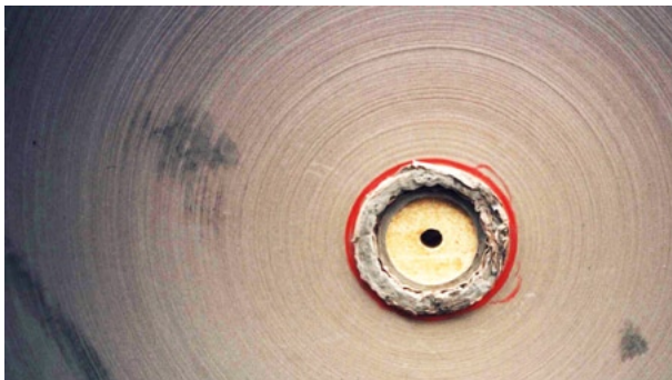
Protruding winding core
