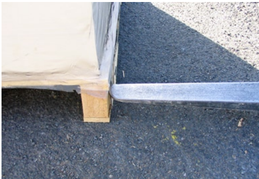
The nails of the pallet foot can tear out
