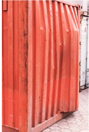
Container wall damaged by the cargo within
