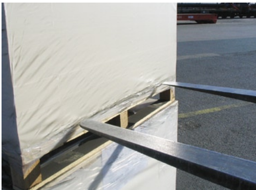
Packaging pierced, damage to paper stack
