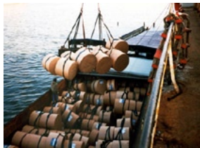
Poor stowage in general cargo vessel
