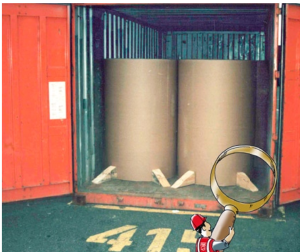
Insufficient blocking / bracing
