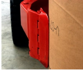
Clamp insufficiently opened
