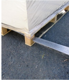
Pallet foot damaged by fork
