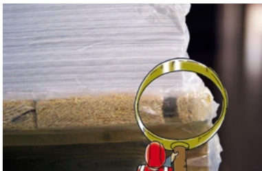
Broken pallet board
