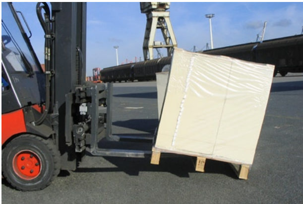
Pallet feet threaten to break off
