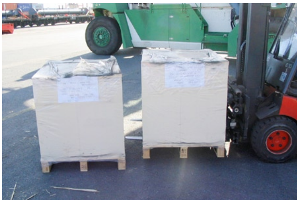
Protruding fork tip penetrates adjacent cargo unit
